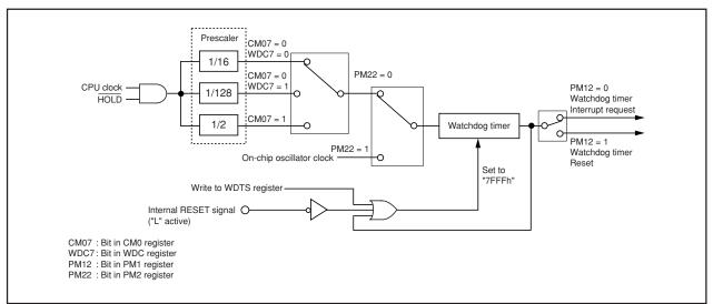
Figure 10.1 Watchdog Timer Block Diagram
